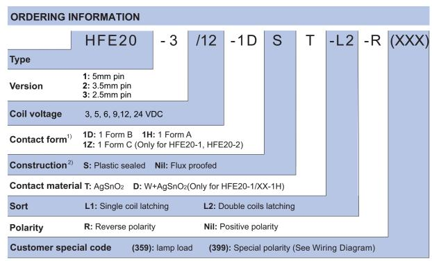
Notes: 1) 1H means that relay is on the "reset" status when delivery; 1D means that relay is on the "set" status when delivery. we will recommend use one form B if customer can use normally (except the pre-make version HFE20-1/XX-1HXD).
