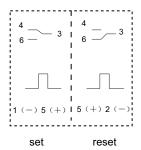
Single coil latching, 1 Form B Double coils latching, 1 Form B
