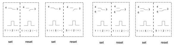
Single coil latching, 1 Form B Double coils latching, 1 Form B
