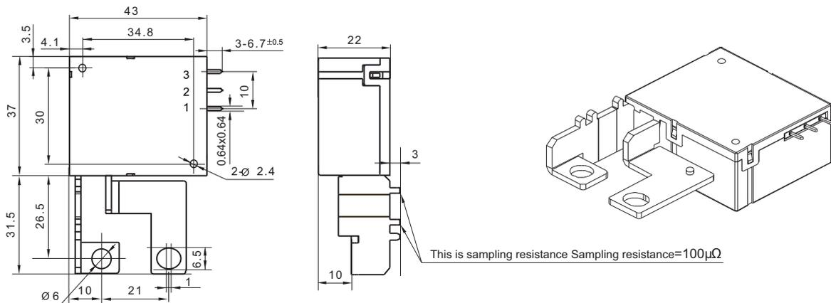
NOTE: The dimension of the load terminals as well as the sampling resistance can be made per customer request.
