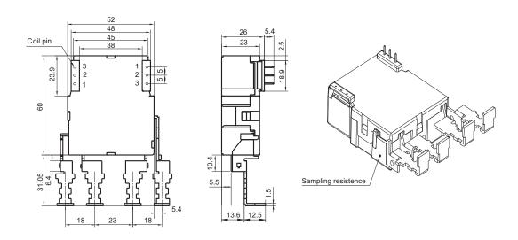
Remark: In case of no tolerance shown in outline dimension: outline dimension ≤1mm, tolerance should be ±0.2mm; outline dimension >1mm and ≤5mm, tolerance should be ±0.3mm; outline dimension >5mm, tolerance should be ±0.4mm.
