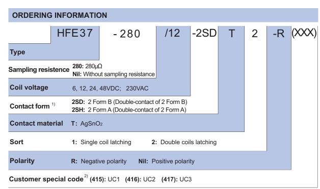
Notes: 1) 2SH means that relay is on the "reset" status when delivery; 2SD means that relay is on the "set" status when delivery. If no speical required by customer, we will keep the relay on the "set" status when delivery.
